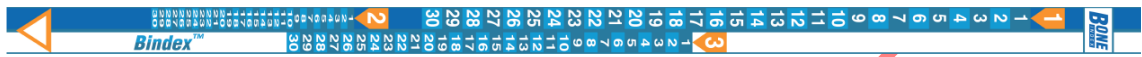
Figure 3: The Bindex Measure is used for determination of standard measurement location at the tibia.
