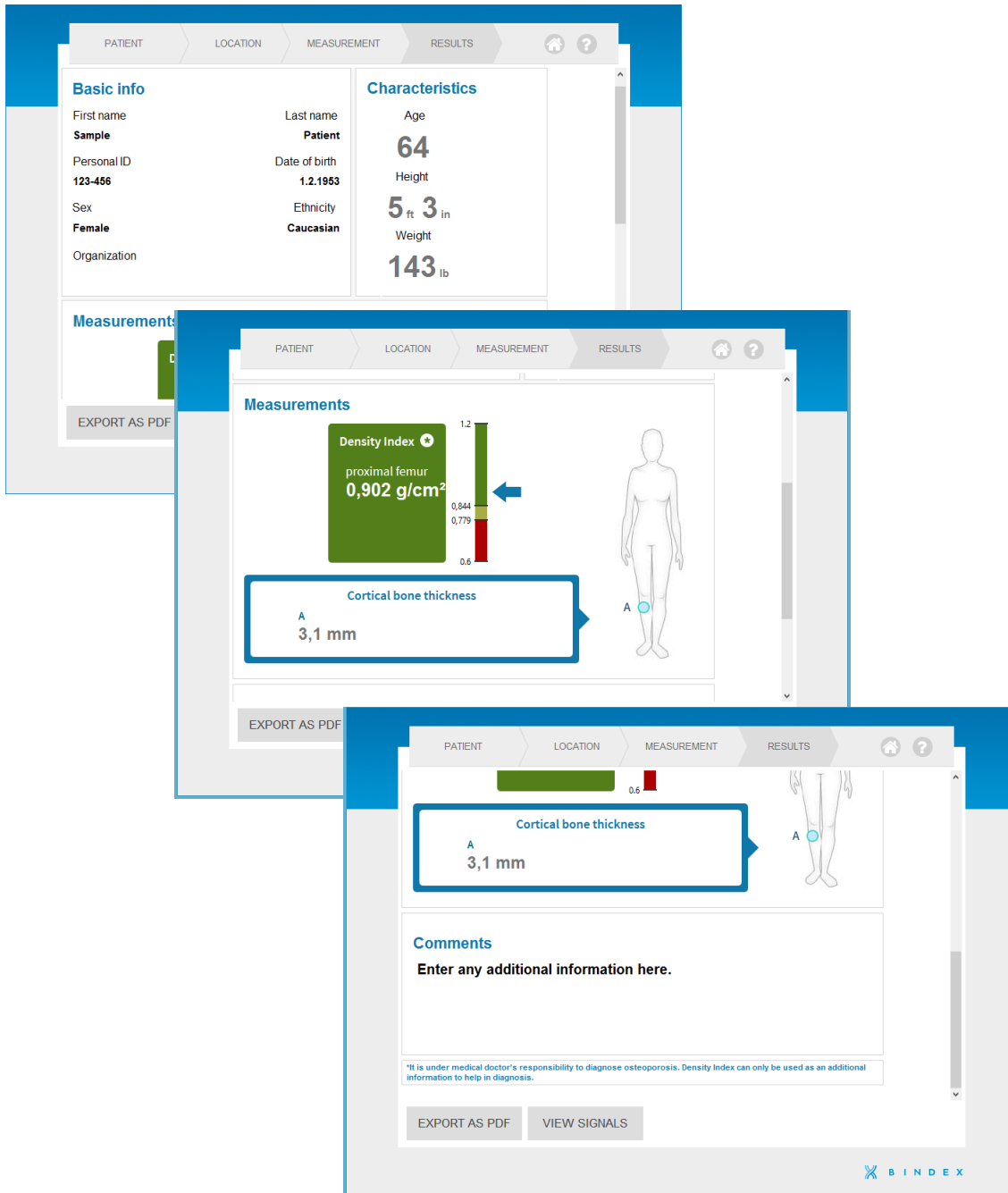
Figure 50: The result page includes patient information, Density Index and apparent cortical bone thickness values. In addition, the Density Index value is also presented on a three-color scale (green, yellow and red).
